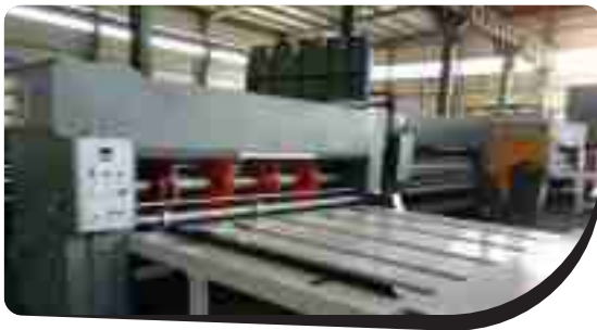
High Speed Corrugation Machine, "B" Flute & "E" "N" Flute
